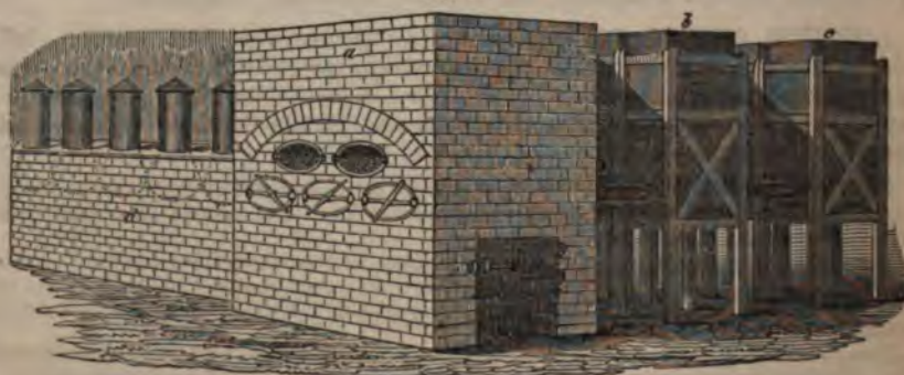
Manufacture of Sesquicarbonate of Ammonia.
